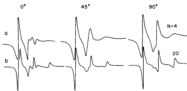
FIG. 8. Calculated ESR spectra with \lambda=3.5 , \rho=-0.6 , R_1=3.8 \times 10^7 \text{ s}^{-1} , T_2^{*-1}=0.7 \text{ G} and (a) N=4 and (b) N=20 , and P(\theta', \phi') \propto (\sin \theta')^{-1} .
