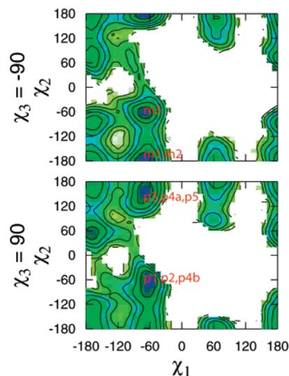
**Figure 9.** The  $\chi_1$ - $\chi_2$  free energy surface computed from the MD trajectories for the two conformations of the disulfide dihedral. The contours correspond to an energy change of 1 kcal/mol. Regions not visited during the simulations are left white.
