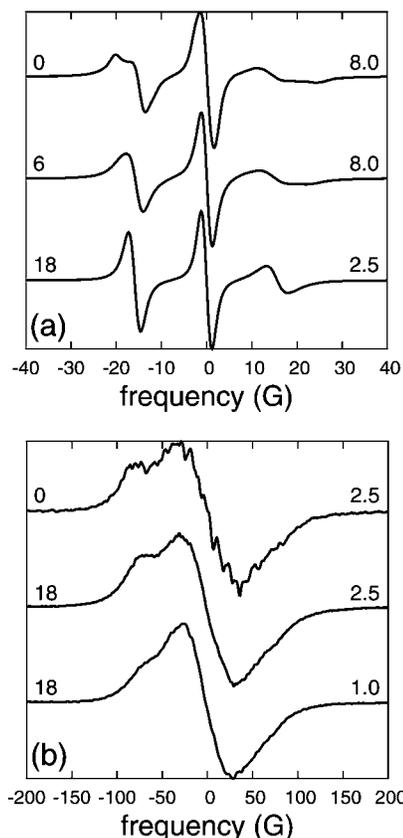
**Figure 12.** (a)  $B = 0.34$  T and (b)  $B = 8.92$  T spectra simulated from the MD trajectories without ( $D = 0$ ) and with ( $D = 6 \times$  and  $18 \times 10^6$  s<sup>-1</sup>) additional tumbling. The diffusion coefficient is indicated on the left, and the scaling factor is indicated on the right-hand side of each spectrum. Other simulation parameters are given in Table 6.
