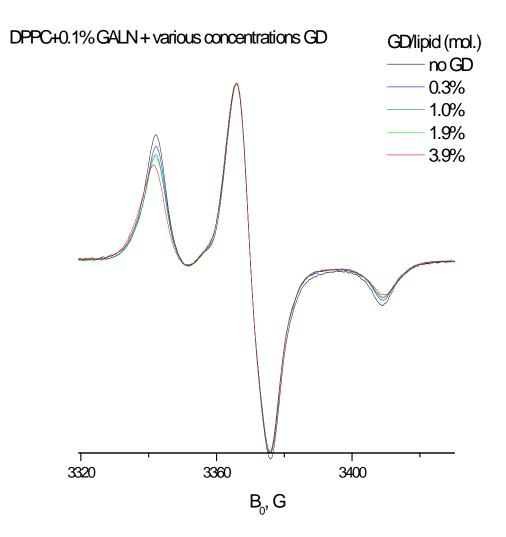
The DHD dimer is long enough to traverse the hydrophobic part of the DPPC membrane (Table 1) so that the spin label reaches the part of the membrane with higher polarity. On the other hand, for GALN monomers the spin label should be located close to the least polar area of the membrane. As seen in the fig, with an increase in the concentration of
