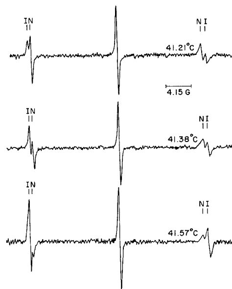
FIG. 1. ESR spectra of PD-tempone in MBBA near T_c = 41.4^\circ\text{C} . The three main lines are due to the hyperfine splitting from a single ^{14}\text{N} nucleus. The peaks marked I and N correspond to isotropic and nematic phases, respectively.
