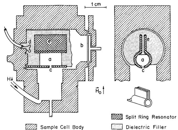
FIG. 2. Left and upper right: Two cross sections through the center of the sample region  $a$ ;  $b$  is the strain gauge,  $c$  is the entrance hole,  $d$  is the coupling loop, and  $e$  is the capacitor. Lower right: perspective view of the resonator, on a smaller scale.
