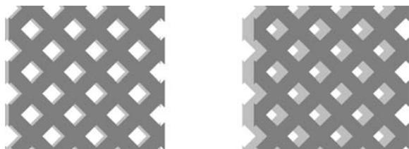
FIG. 6. Variable coupling arrangement. By shifting stacked inductive meshes relative to each other, the effective hole size and the reflectivity can be adjusted. The square shape of the holes is maintained and ensures the existence of orthogonally polarized degenerate resonator modes used for excitation and detection.
